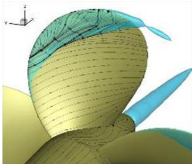
Figure 1 - Ship propeller cavitation CFD simulation
